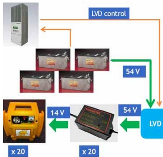
Figure 6b: System Load Schematic to Home Packs
