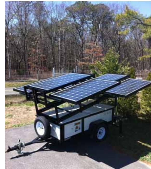
Figure 3: SunBlazer in Production Mode, Station & Home Batteries & Controls Secured
