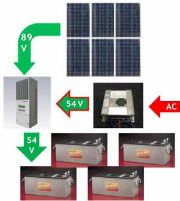
Figure 6a: PV Solar & Optional Auxiliary AC Station Battery Charging Circuits
