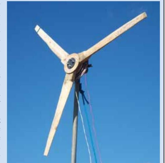
Figure 10. 700W Wind Turbine Prototype Under Test in Zambia
