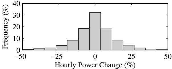
Fig. 2. Normalized histogram of the hour-to-hour variation in wind power.
