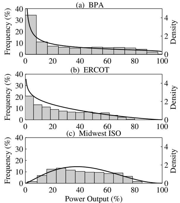
Fig. 3. Normalized histograms of the wind power in each data set with corresponding fit Beta distributions.
